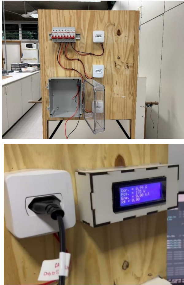
Figure 12 – Image of the wooden panel and the power box (left), as well as the display. LCD to display real-time readings (right).
