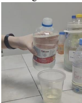
Figure 2: Adding an Organic Solvent (646)
