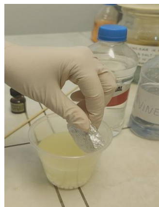
Figure 3: Dissolving EPS foam plastic in the solvent blend.
